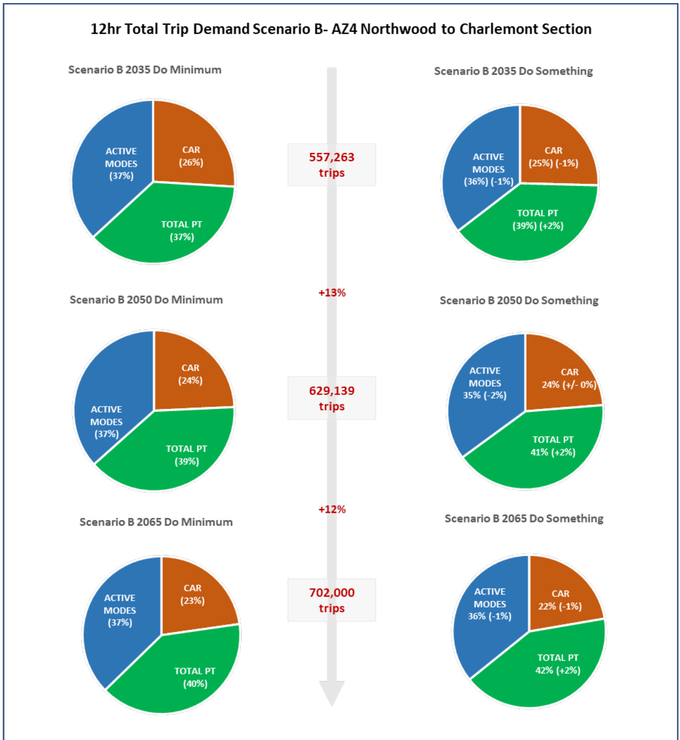
Diagram 9.63: Scenario B 12hr Peak Period Total Trip Demand – AZ4 Northwood to Charlemont Section
